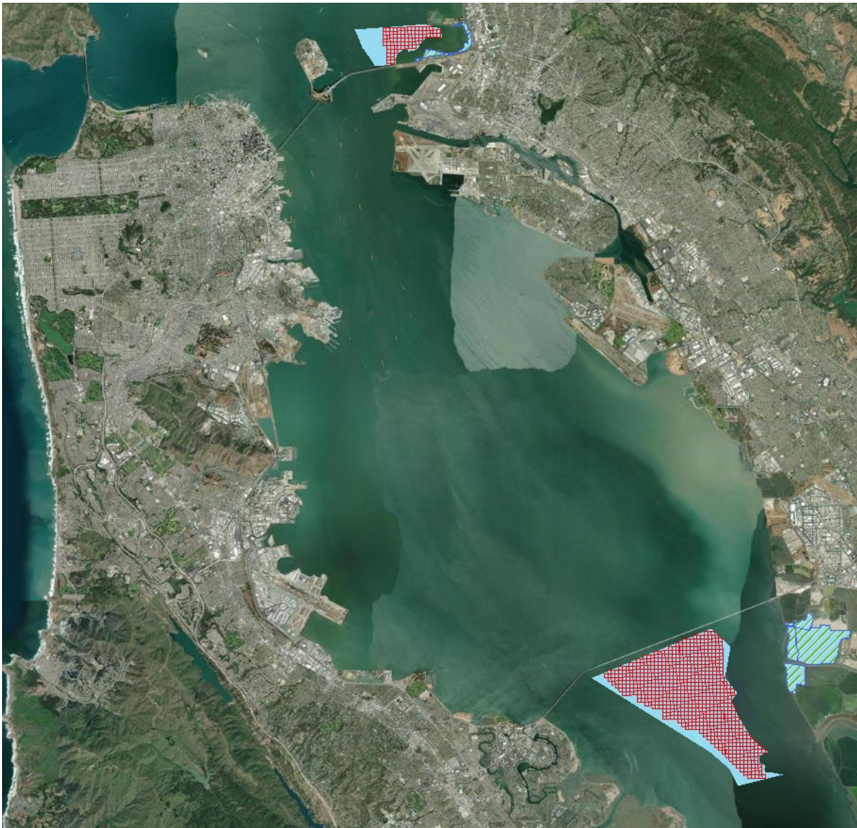
Figure 5. Strategic placement sites narrowed down from twelve to two: Emeryville (top) and Eden Landing (bottom). Site map includes both placement footprint (red grid) and target marsh for restoration (aqua hatch).
